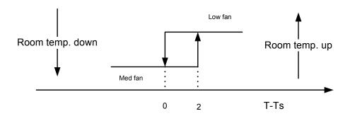
8.7.6 Indoor evaporator high-temperature protection at heating mode (T=indoor exchanger temp.)
